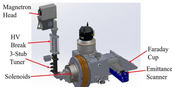
Figure 2: CAD model of the test stand.
