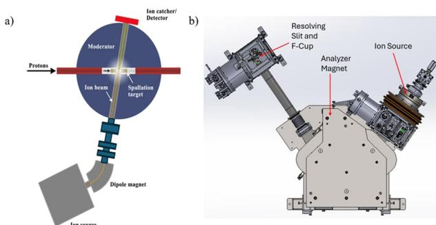
Figure 1: a) Schematic of the NTD project. Figure provided by A. Cooper at LANSCCE under LA-UR-24-27491. b) Plan view of the CAD model for the ion source system.
