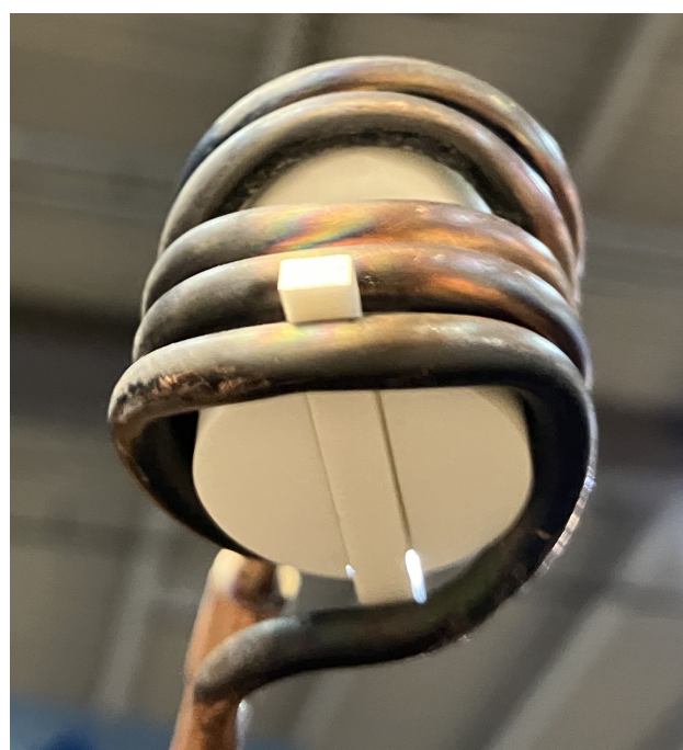
Figure 3: Inductive oven viewed from below. The support post rests on the bottom turn of the coil and a slot in the insulator prevents rotation of the insulator relative to the coils.
