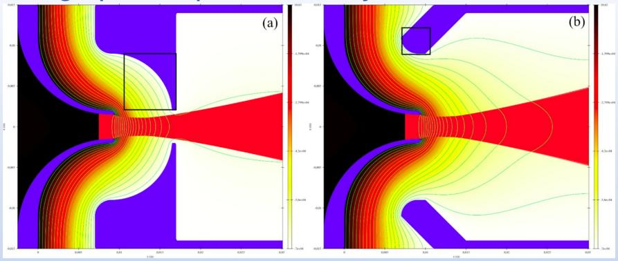
Despite the native transverse E-field, the spherical extractor may enhance the beam divergence due to lower influence of the space charge.
