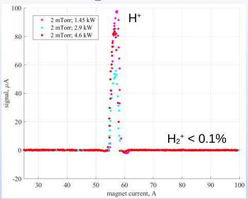
Pure proton beam with no need to separate
