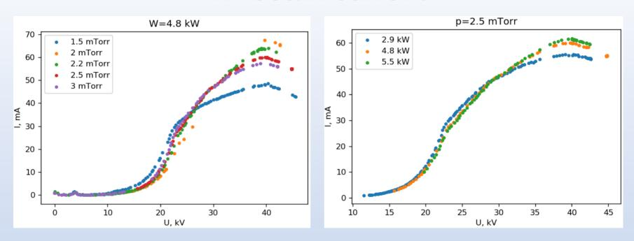
In combination with intrinsic magnetic lenses, the spherical extractor allowed us to achieve >60 mA of H+ beam at 40 keV. Beam size (>99%) is 50 mm at 70 cm from the extraction system. Yet >100 mA are lost in the beam line (puller) and may be delivered with the enhanced multi-electrode beam forming configuration.
