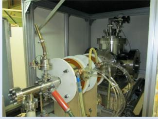
Frequency 37.5 or 75 GHz Power up to 100 kW Pulse duration 1 ms Trap magnetic field up to 5 T
