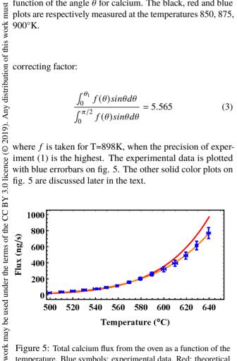
Figure 5: Total calcium flux from the oven as a function of the temperature. Blue symbols: experimental data. Red: theoretical data with  $S = s + s_c$  and Ca data from [4]. Orange: least mean square fit of experimental data using  $S = s + s_c$  and Antoine's law (see. Eq. 4) coefficients A and B as fit parameters
