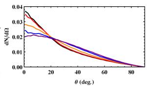
Figure 6: Normalized differential distribution of atoms at the exit of the oven per unit of solid angle as a function of  $\theta$  for different temperatures: 600K (black), 900K (red), 1000K (orange), 1100K (blue), 1200K (purple).
