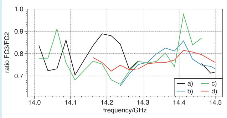
This seems to indicate that the beam emitted from the source occupies a different volume (size and/or shape) in phase space for the different microwave frequencies It was not possible to measure the emittance directly. It is known that the transmission through the LEBT and the RFQ is sensitive concerning changes of the beam energy.
