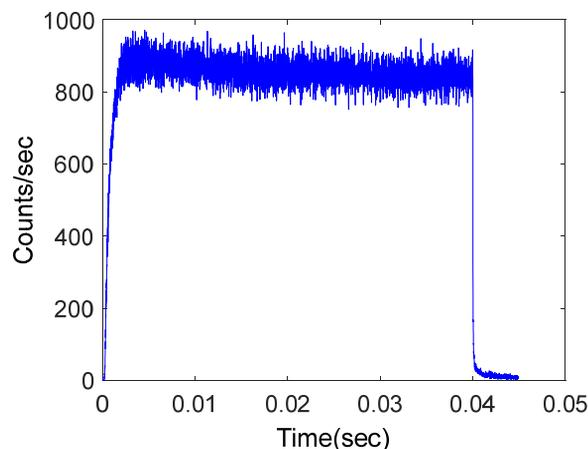
Figure 5: X-ray emission rate as function of time at 6.83 GHz and  $B_{min}/B_{ECR}=0.95$ .
