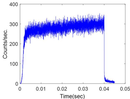
Figure 6: X-ray emission rate as function of time at 6.83 GHz and  $B_{min}/B_{ECR}=1.01$ .
