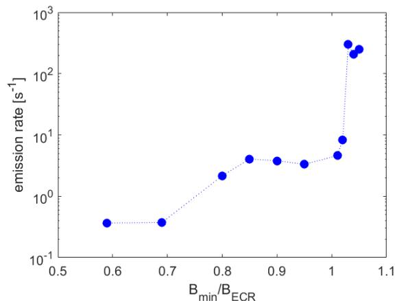
Figure 4: X-ray emission rate versus different simple mirror configurations at 4.1 GHz.
