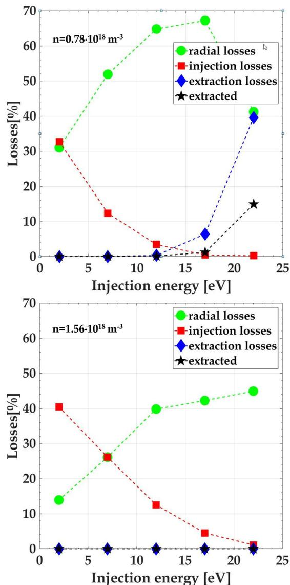
Figure 2:  $^{85}\text{Rb}^{1+}$  ions losses in different directions as a function of the injection energy for  $KT_i=0.5$  eV,  $n=1.56\cdot 10^{18}$   $\text{m}^{-3}$  (bottom) and  $n=0.78\cdot 10^{18}$   $\text{m}^{-3}$  (top). The directions considered are radial (green), back to the injection side (red), towards the extraction end plate (blue) and the one passing through the 7 mm diameter extraction hole of the Charge Breeder (extracted).
