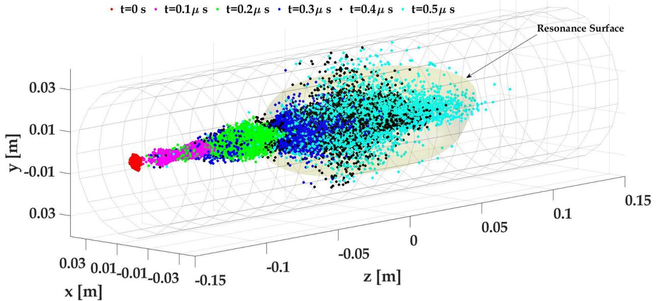
Figure 3: Plot of the injected particles trajectories at different time steps for an injection energy of 7 eV:  $t=0 \mu\text{s}$  (red),  $t=0.1 \mu\text{s}$  (magenta),  $t=0.2 \mu\text{s}$  (green),  $t=0.3 \mu\text{s}$  (blue),  $t=0.4 \mu\text{s}$  (black),  $t=0.5 \mu\text{s}$  (cyan). The cylinder represents the Charge Breeder plasma chamber, while the egg-shaped surface indicates the resonance surface containing the plasmoid.
