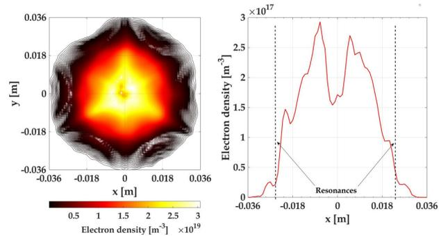
Figure 5: Density plots obtained after two steps of the self-consistent loop: projection on the  $xy$  plane (left) and radial profile along the  $x$  axis in the midplane (right).
