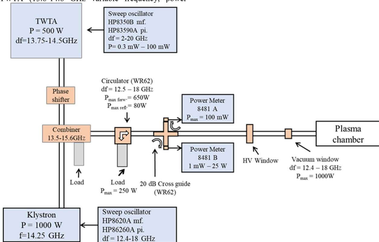
Figure 4: The microwave coupling system to study the two-close-frequency operation mode in ECR ion sources.
