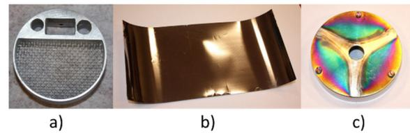
Figure 2: New materials in the plasma chamber. a) Injection plate, aluminum, mesh transparency is 60%. b) Lateral wall is tantalum. c) Plasma electrode covered with titanium.
