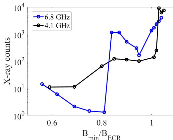
Figure 3: X-ray emission rate versus different simple mirror configurations. For both the frequencies, the pressure and the absorbed power are  $8 \cdot 10^{-5}$  mbar and 80 W, respectively.
