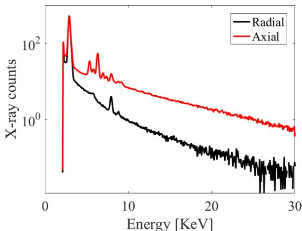
Figure 5: Typical x-rays spectra acquired by Si-Pin from axial and radial ports. Fluorescence lines of Ar and Cu are visible in both spectra. The pressure and the absorbed power are  $8 \cdot 10^{-5}$  mbar and 80 W, respectively.
