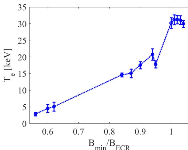
Figure 4: The dependence of  $T_e$  versus different simple mirror configurations.
