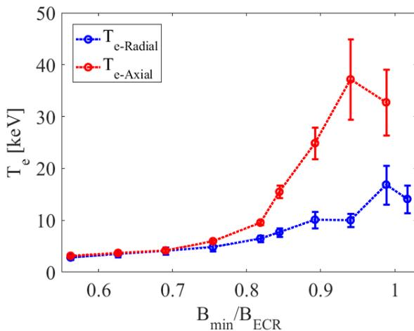
Figure 8: The dependence of  $T_e$  versus different simple mirror configurations.
