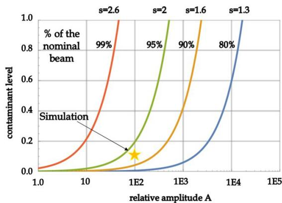
Figure 5: Expected contamination as a function of the relative amplitude  $A=I_{non-nom}/I_{nom}$  between the non-nominal and the nominal beam for different values of  $s$  and  $d=4$ . Simulations gave better results compared to the estimation made considering the gaussian shape of the two peaks.
