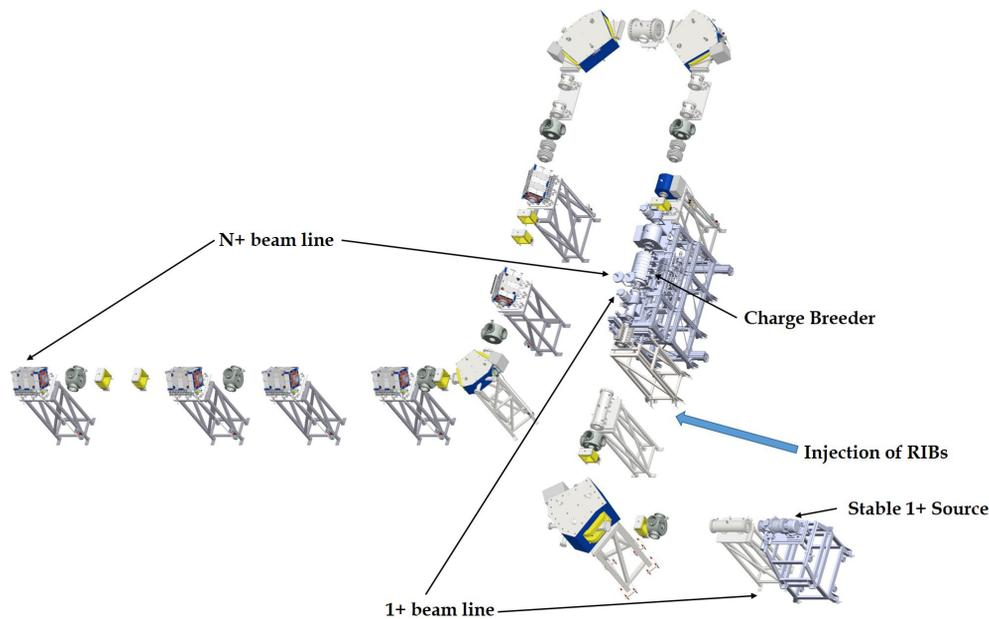
Figure 1: Prospective view of the ADIGE injector with its 1+ beam line (from the 1+ Source to the Charge Breeder) and N+ beam line (from the Charge Breeder on). The position where the 1+ beam line for RIBs will be connected is also shown.
