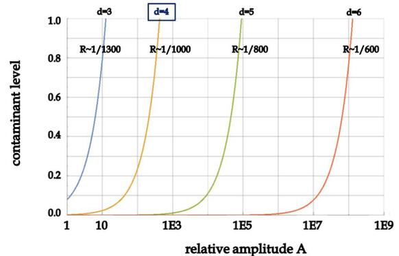
Figure 4: Expected contamination as a function of the relative amplitude  $A=I_{non-nom}/I_{nom}$  between the non-nominal and the nominal beam for different values of  $d$  and  $s=d/2$ ; the MRMS corresponds to  $d=4$ .
