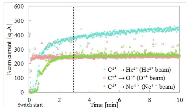
Figure 6: Switching time of He<sup>2+</sup>, O<sup>3+</sup> and Ne<sup>4+</sup> from C<sup>2+</sup>.
