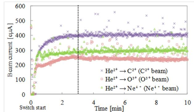
Figure 5: Switching time of C<sup>2+</sup>, O<sup>3+</sup> and Ne<sup>4+</sup> from He<sup>2+</sup>.
