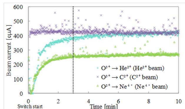
Figure 7: Switching of He<sup>2+</sup>, C<sup>2+</sup> and Ne<sup>4+</sup> from O<sup>3+</sup>.
