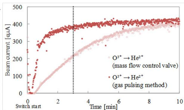
Figure 4: Reproducibility of He<sup>2+</sup> at the switching of O<sup>3+</sup> with mass flow control valve and gas pulsing method.
