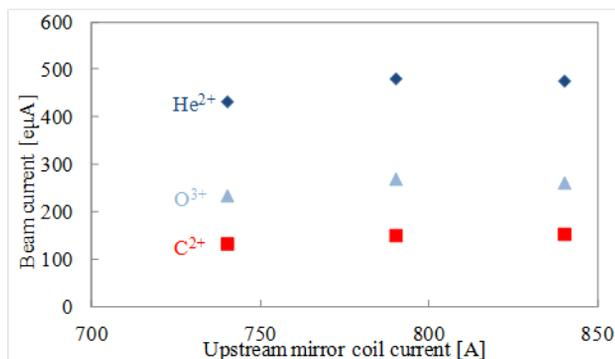
Figure 2: Dependence of upstream mirror magnetic field.
