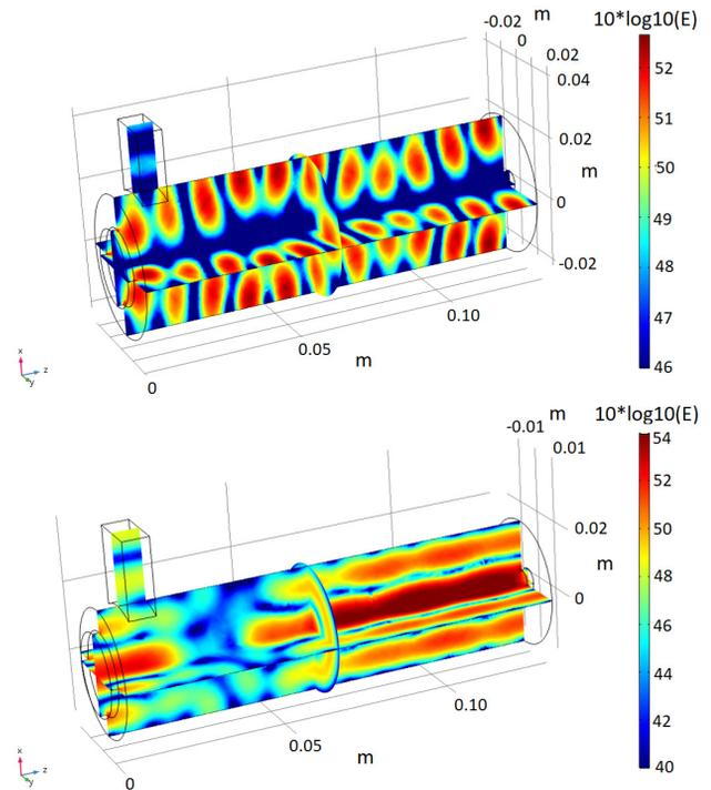
Figure 4: Electric field distribution in logarithmic scale calculated through the COMSOL<sup>®</sup> frequency domain solver: 14.428 GHz for the present chamber (top), 14.395 GHz for the modified chamber (bottom).
