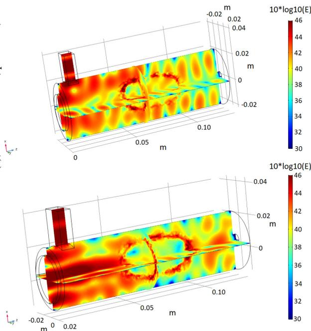
Figure 5: Electric field distribution in logarithmic scale calculated through the COMSOL<sup>®</sup> frequency domain solver and including the plasma: 14.428 GHz for the present chamber (top); 14.395 GHz for the modified chamber (bottom).
