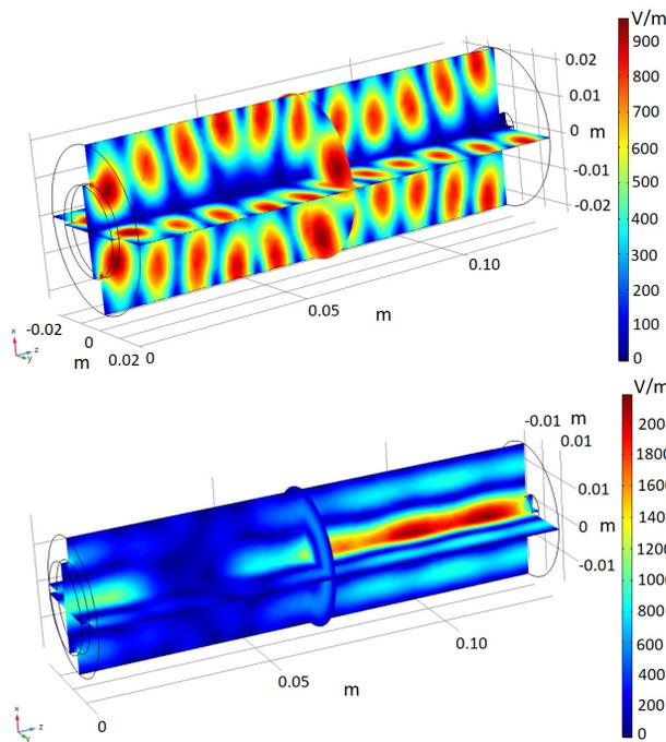
Figure 3: Electric field distribution calculated through the COMSOL<sup>®</sup> eigenmode solver including the injection and extraction holes: the present chamber with the TE<sub>2,1,11</sub> mode shifted at 14.428 GHz (top); the modified chamber with the TM<sub>0,2,0</sub> shifted at 14.432 GHz (bottom).
