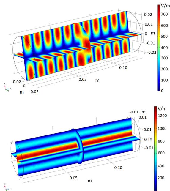
Figure 2: Electric field distribution calculated through the COMSOL® eigenmode solver: the present chamber with the  $TE_{2,1,11}$  mode (top), the modified chamber with the  $TM_{0,0,2}$  (bottom).
