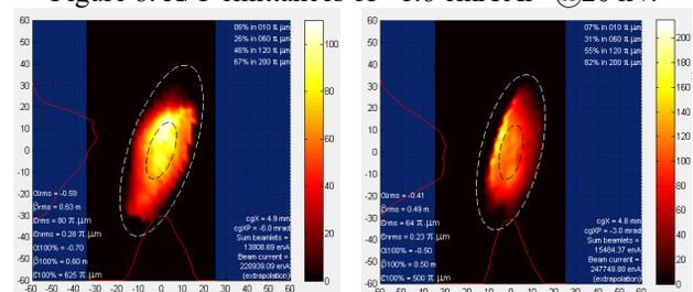
Figure 7: X/Y emittances of ~0.7 emA Ar<sup>12+</sup>@20 kV.
