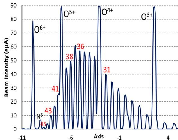
Figure 2: Production of high charge Xe beams.
