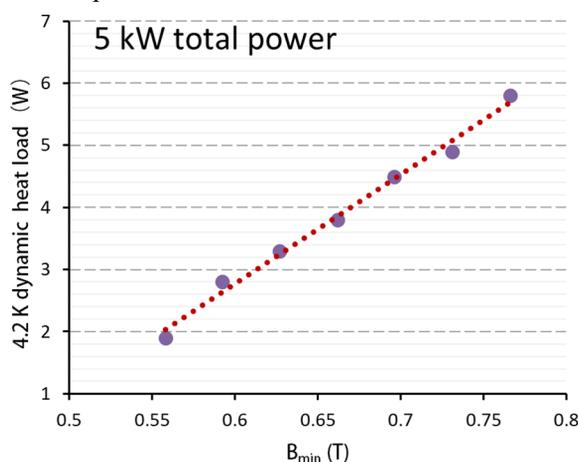
Figure 4: Dynamic heat load vs.  $B_{\text{min}}$  with SECRAL-II.
