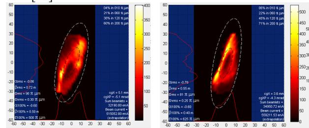
Figure 6: X/Y emittances of ~1.6 emA Ar<sup>9+</sup>@20 kV.
