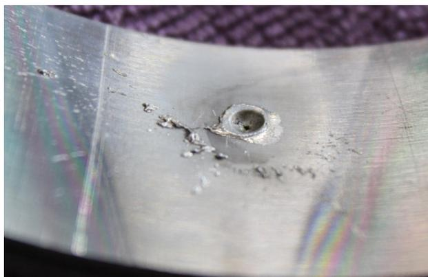
Figure 3: Sectional burnt-out chamber wall.
