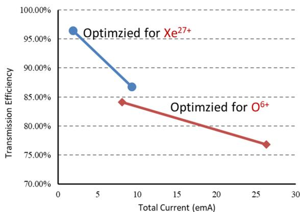
Figure 5: Beam transmission efficiency with SECRAI-LEBT at different total beam intensities.
