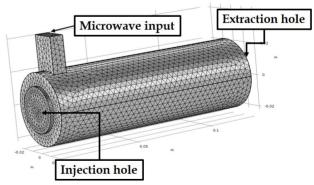
Figure 1: Model of the plasma chamber of the LEGIS source implemented in COMSOL<sup>®</sup>. Microwaves are injected through a radial rectangular WR62 waveguide. The extraction hole is not visible.
