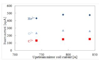
Figure 2: Dependence of upstream mirror magnetic field.
