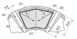
Figure 1: A through cut of a section of the aluminium hexapole container including the canned magnet bar, (a) pumping ports, (b) pumping holes, (c) loss-lines, (d) space filled with SS sheets, (e) can, (f) easy axis.
