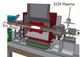
Figure 2: Schematic of the new 28-GHz SC-ECRIS.
