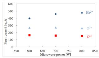
Figure 1: Dependence of microwave power.
