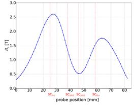
Figure 1: AISHa magnetic field profile
