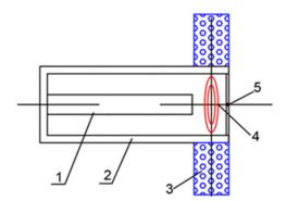
Figure 3: Schematic structure of the ECR ion source based on a coaxial resonator. 1 - central conductor of a coaxial resonator; 2 - resonator casing; 3 - magnetic
