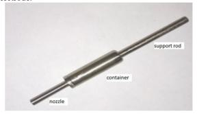
Figure 1: The large volume crucible.
