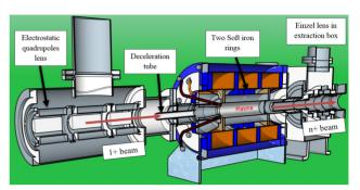
Figure 1: 3D view of ECR charge breeder connected with injection and extraction systems.
