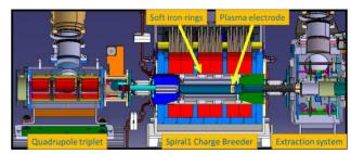
Figure 1: SPIRAL1 Charge Breeder.
