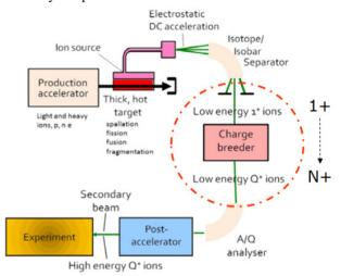
Figure 1: Layout of isotope online (ISOL) accelerator.
