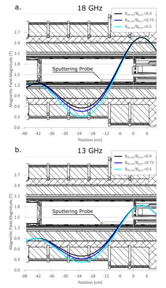
Figure 1: SuSI Magnetic field as simulated using Poisson with the radial sputtering probe developed for SuSI (dotted line). Three field configurations:  $B_{min}/B_{ecr}=0.5, 0.73$ . and 0.9 were selected for both 18 GHz and 13 GHz operation. The magnetic fields were scaled with frequency resulting in the same ECR zone size for constant  $B_{min}/B_{ecr}$  ratio. The radial sputtering probe was inserted in between the electron flutes on the injection baffle along the plasma chamber wall.
