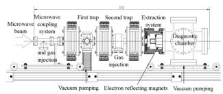
Figure 1: The scheme of the experimental facility.
