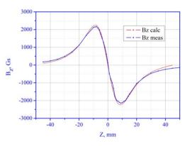
Figure 1: Axial magnetic field distribution of a ring magnet.
