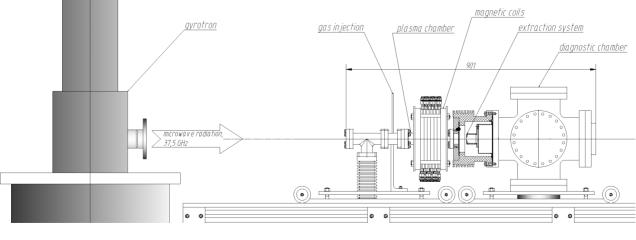
Figure 1: The experimental facility SMIS 37.
