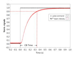
Principle of Figure 1: the traditional  $\tau_{CB}$ measurement. The dashed lines are the references of the pulse start (black) and 90% level of the Rb<sup>20+</sup> beam intensity (red).
