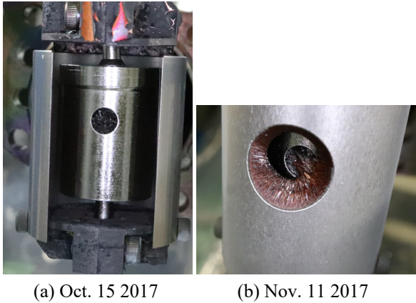
Figure 5: Blockage of the vapor-ejection hole of crucibles.
