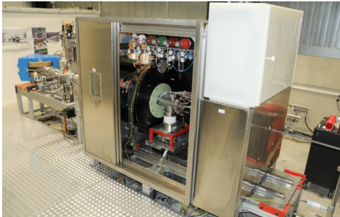
Figure 2: The Advanced Ion Source for Hadrontherapy at INFN-LNS in Catania.
