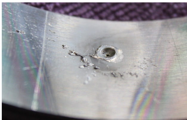
Figure 3: Sectional burnt-out chamber wall.
