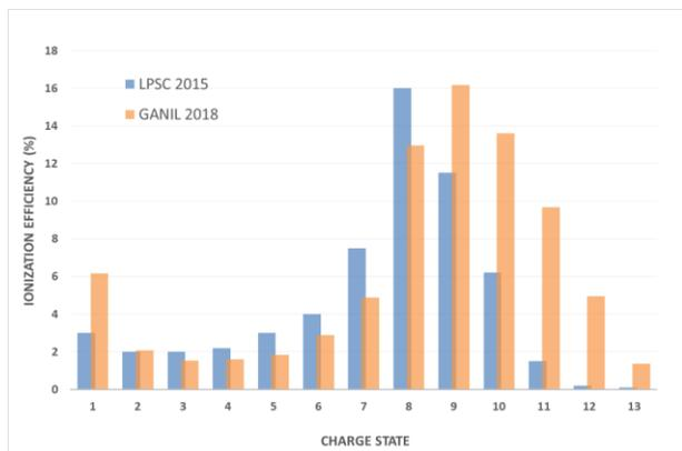
Figure 2:  $^{40}\text{Ar}^{q+}$  charge state distributions.
