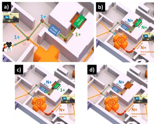
Figure 3: Four modes available at SPIRAL1 facility. a) Shooting through 1+ b) Shooting through N+ c) 1+/N+ d) SP1 CB as injector.
