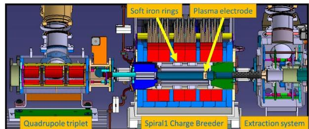
Figure 1: SPIRAL1 Charge Breeder.
