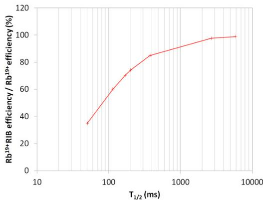
Figure 7: Evolution of the  $\text{Rb}^{19+}$  RIB efficiency over  $\text{Rb}^{19+}$  stable efficiency ratio as a function of  $T_{1/2}$ .
