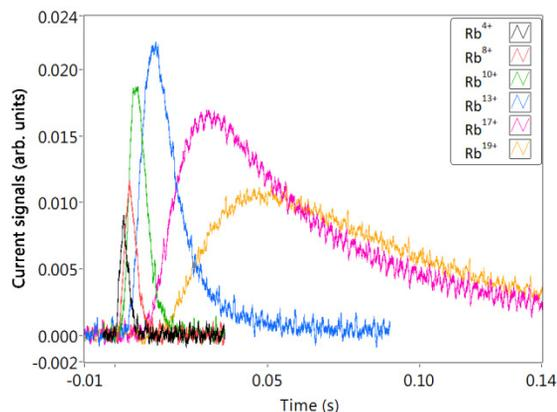
Figure 4: Rb<sup>4+</sup>, Rb<sup>8+</sup>, Rb<sup>10+</sup>, Rb<sup>13+</sup>, Rb<sup>17+</sup> and Rb<sup>19+</sup> beam intensity responses to a 2.5 ms injection pulse.
