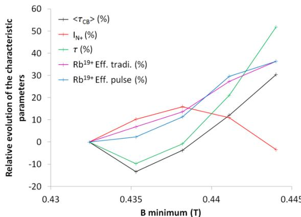
Figure 6: Variation of the time characteristics, maximum current and Rb<sup>19+</sup> efficiency as a function of the median axial field.
