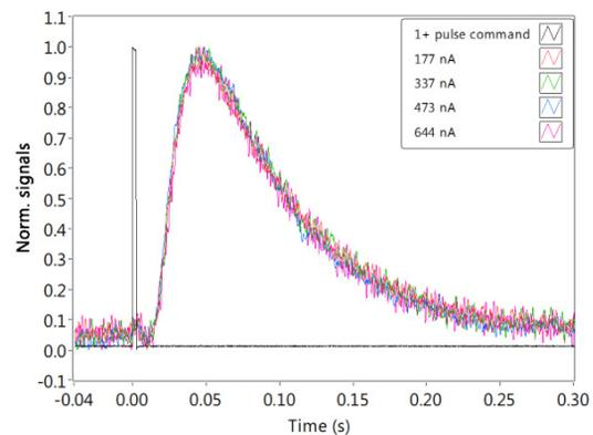
Figure 3: 1+ injection pulse and Rb<sup>19+</sup> normalized signal responses to several 1+ beam pulse intensities.
