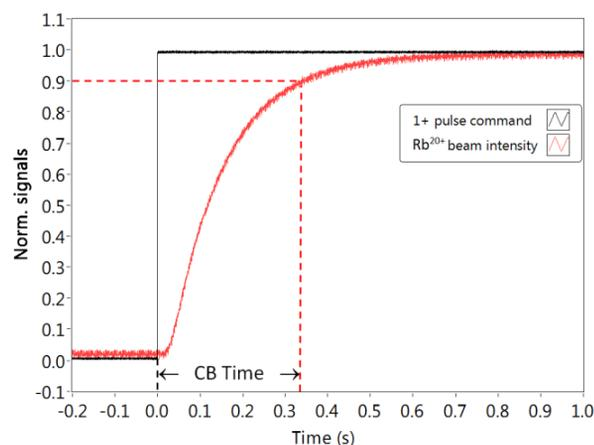
Figure 1: Principle of the traditional  $\tau_{CB}$  measurement. The dashed lines are the references of the pulse start (black) and 90% level of the Rb<sup>20+</sup> beam intensity (red).
