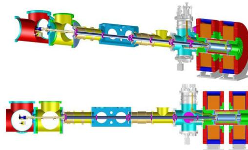
Figure 6: 2.5 meter SPIG joining LIG to CB-ECRIS.
