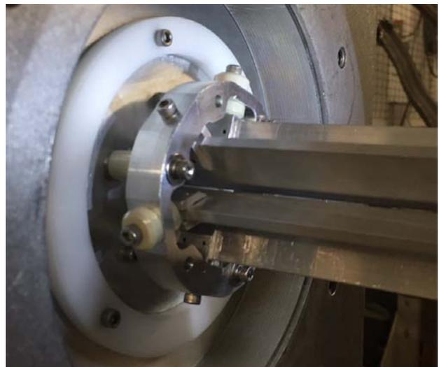
Figure 7: Vaned SPIG and pumping baffle.
