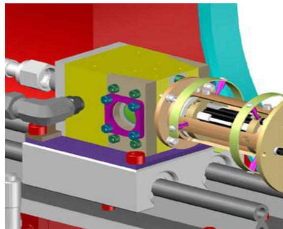
Figure 3: The target-cell and first SPIG section.
