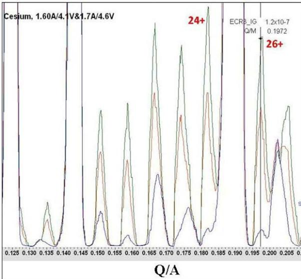
Figure 5: Spectrum of charge-bred Cs. The red and green peaks are Cs charge-states resulting from different 1+ source power levels. The blue is background. 370 enA full scale.
