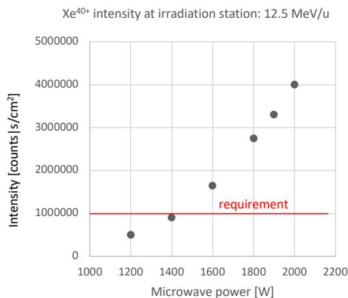
Figure 3:  $Xe^{40+}$  particle intensity (12.5 MeV/u) on the irradiation target as a function of the microwave power. The red horizontal line shows the intensity requirement.
