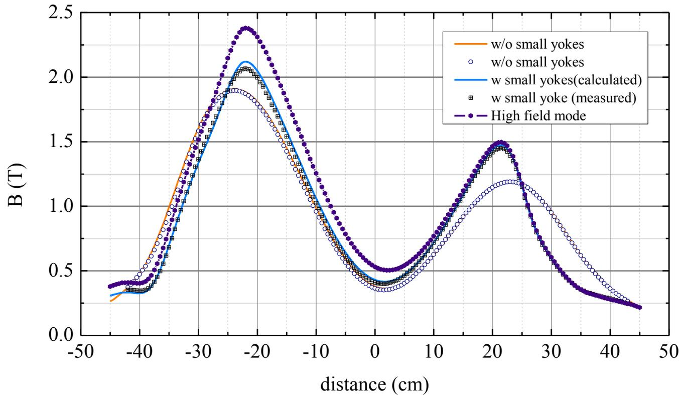
*B-field profiles from the new fast ramping SC magnet II*
