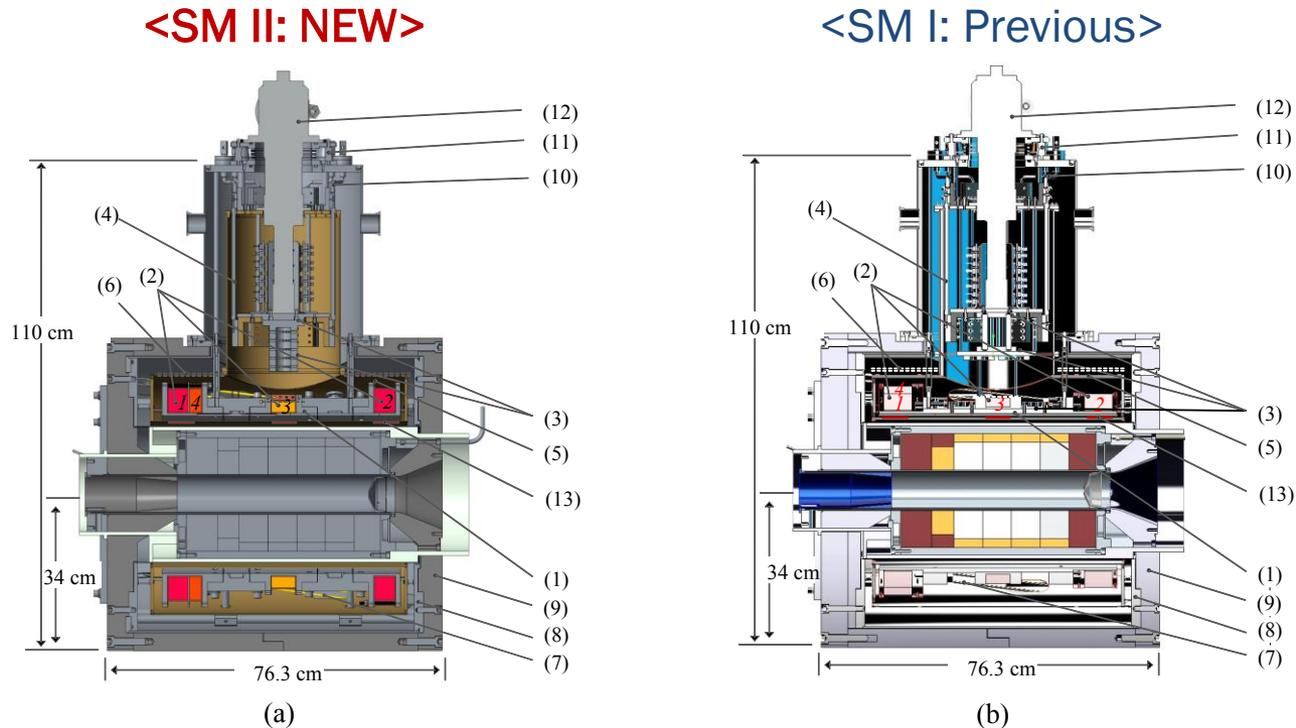
(a) A newly-upgraded SC magnet capable of fast-ramping & higher magnetic field compared with the previous SC magnet:
