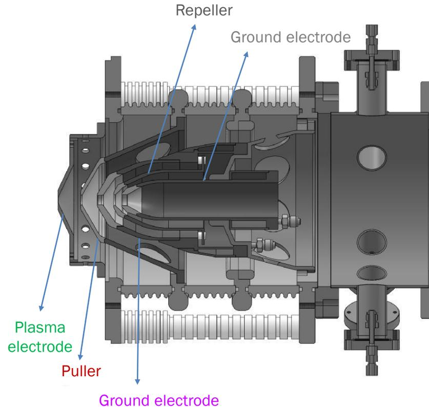
**Pentode (5-electrode) extraction** (based on the extraction structure of Saclay/CEA source)
