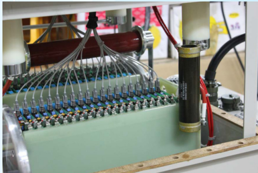
Semiconductor switch (push-pull type, 80 IGBTs connected in series)
