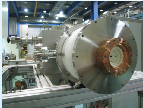
4. Install an plasma chamber
