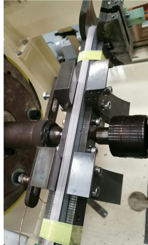
\text{Nb}_3\text{Sn} Sextupole coil winding
