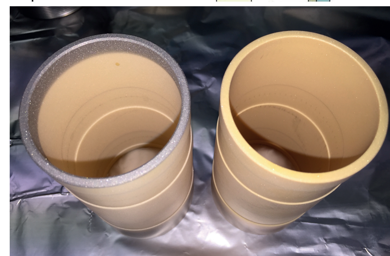
The top part of the figure shows the position of the insulator and the side of the metallization. The electrodes from left to right: plasma electrode (purple), intermediate electrode (yellow) and ground electrode (grey). In the lower part of the figure the left insulator shows a clear metallization on the top after around 6 months of argon beam operation. The right lower part shows for comparison an insulator that was used around 8 months during lead beam operation.
