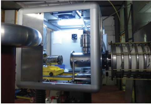
Figure 7: 5.8 GHz ion source mounted on the 250 kV platform of GENEPI2.
