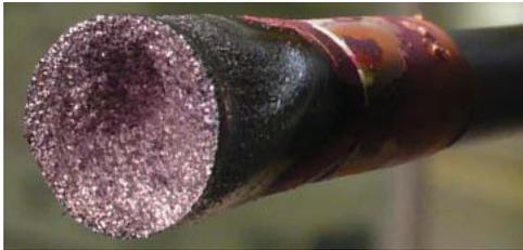
Figure 5: Aspect of the Ta electrode after the 17 days run.
