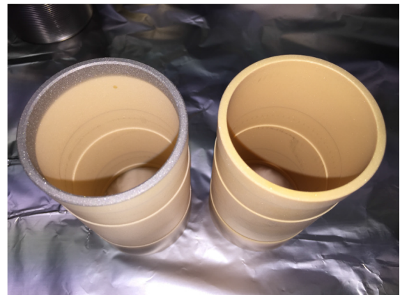
Figure 3: The insulator between the extraction electrodes. The top part of the figure shows the position of the insulator and the side of the metallization. The electrodes from left to right: plasma electrode (purple), intermediate electrode (yellow) and ground electrode (grey). In the lower part of the figure the left insulator shows a clear metallization on the top after around 6 months of argon beam operation. The right lower part shows for comparison an insulator that was used around 8 months during lead beam operation.
