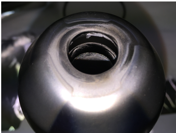
Figure 2: Tip of the intermediate electrode with clear signs of erosion.
