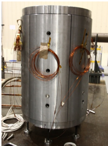
Figure 4: Completed cold mass at the assembly site.
