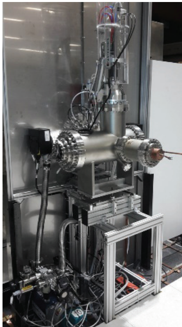
Figure 3: LEBT configuration for the first two beam commissioning phases.
