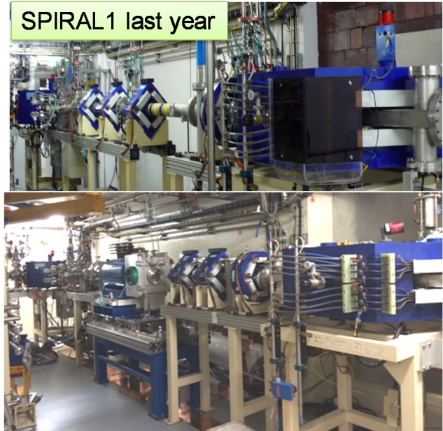
Figure 8: Top: low energy beam line before modifications Bottom: low energy beam line after inclusion of the Spirall charge breeder.
