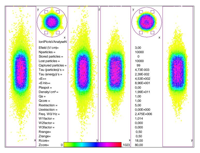
The rotational energies <E> reproduce the resonance dips of He+ they increase up to about 12 V/cm and then saturate The ions with high <E> are concentrated in the resonance volume in perfect agreement with our interpretation that E<sub>rot</sub> reduces the extraction
