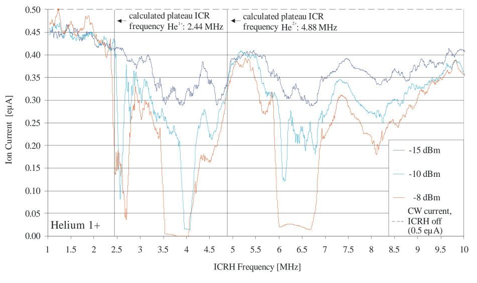
RF is varied in steps of 100 kHz from 1 to 10 MHz at B = 0.64 T
