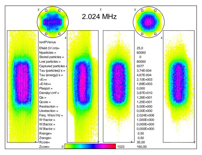
ICRH of Ar5+ at 1.062 T, i.e. 62.7 % above the central  $B_{min}$  of VENUS <E> = 1 keV,  $E_{max}$  = 9.9 keV, <tau> = 0.36 ms, and tau<sub>max</sub> = 11 ms
