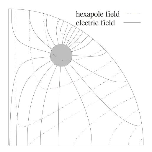
The electric field can penetrate where the electric field  $\perp$  hexapole field
