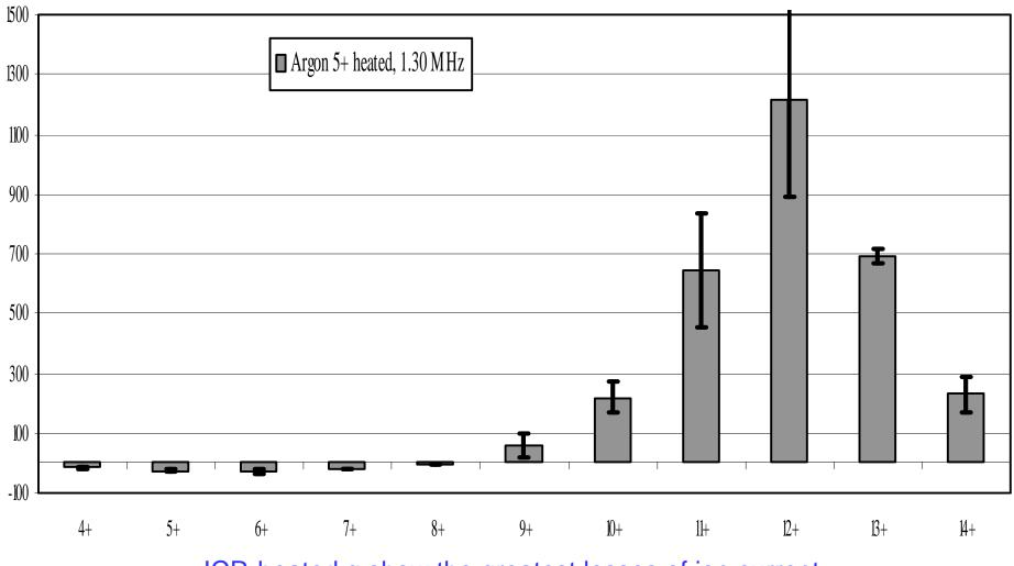
ICR-heated q show the greatest losses of ion current
