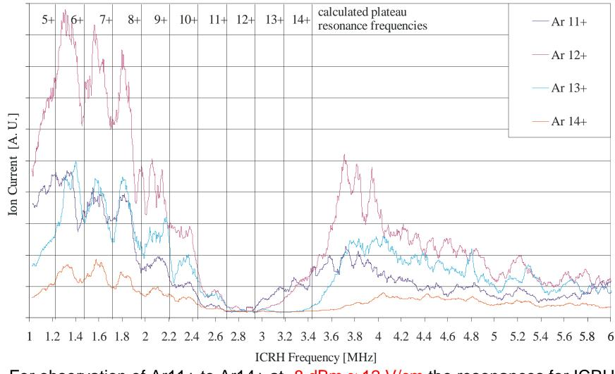
For observation of Ar11+ to Ar14+ at -8 dBm ≈ 12 V/cm the resonances for ICRH
