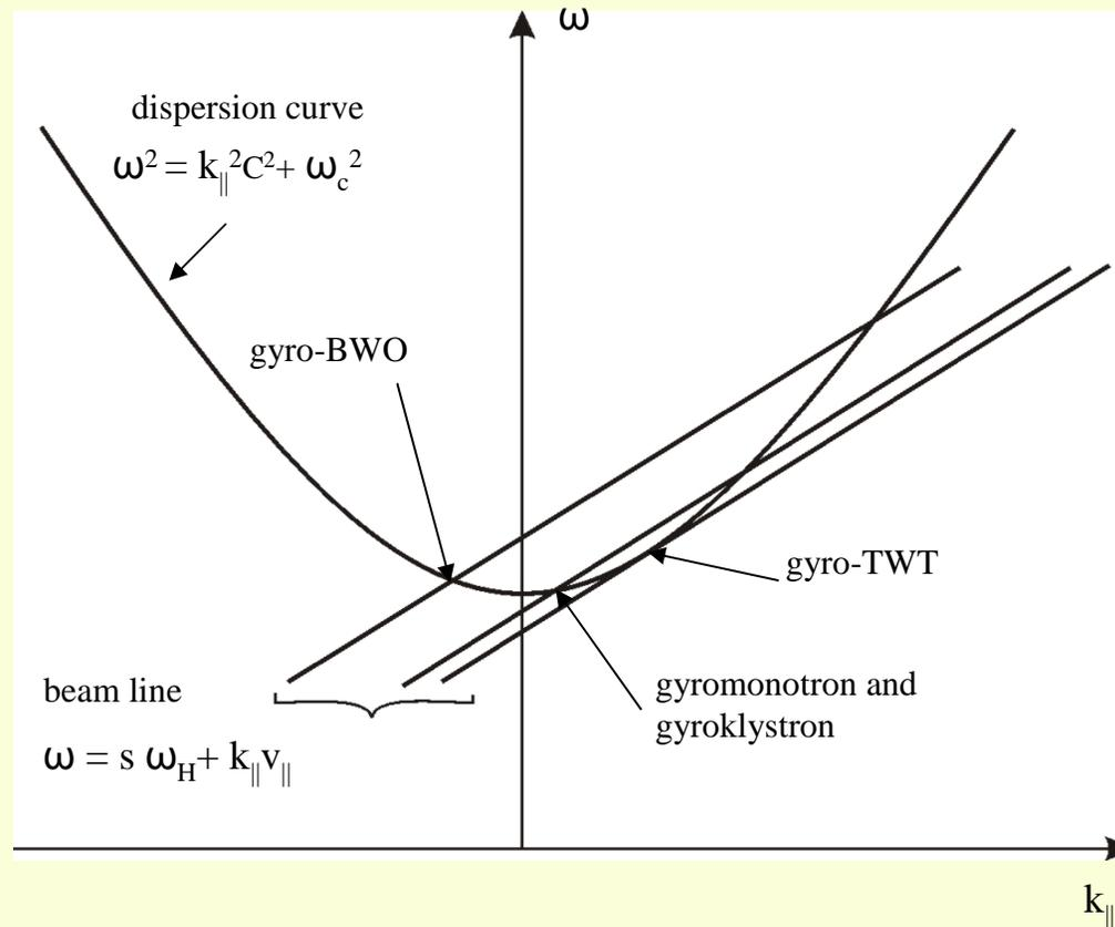
Dispersion diagram showing the operating point for gyro-devices:
