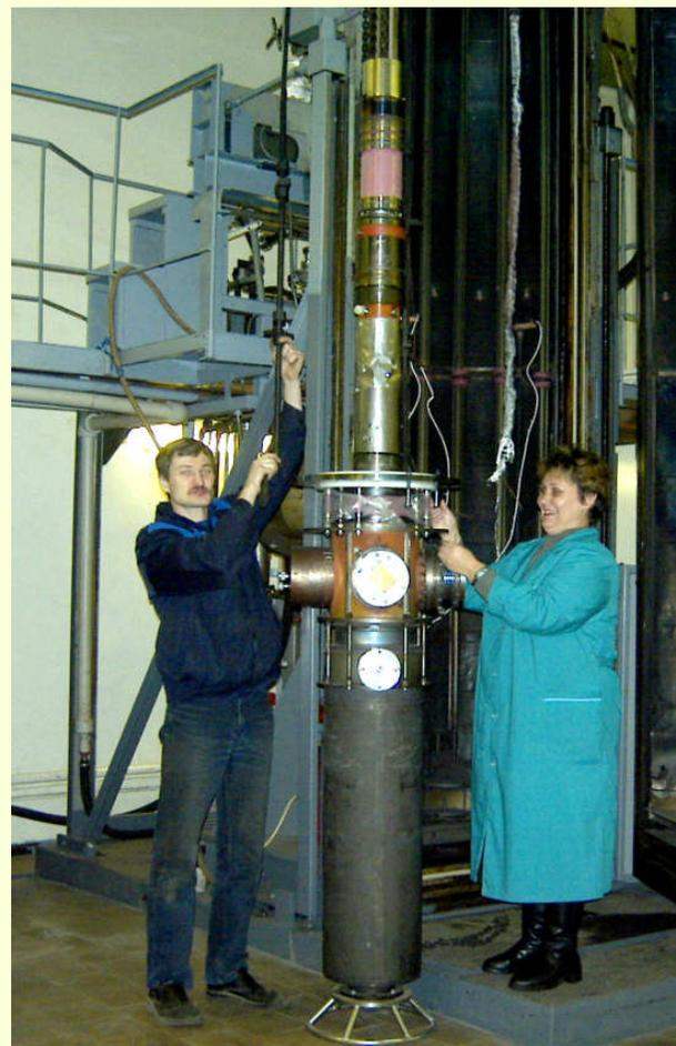
Gyrotron for ITER under development
