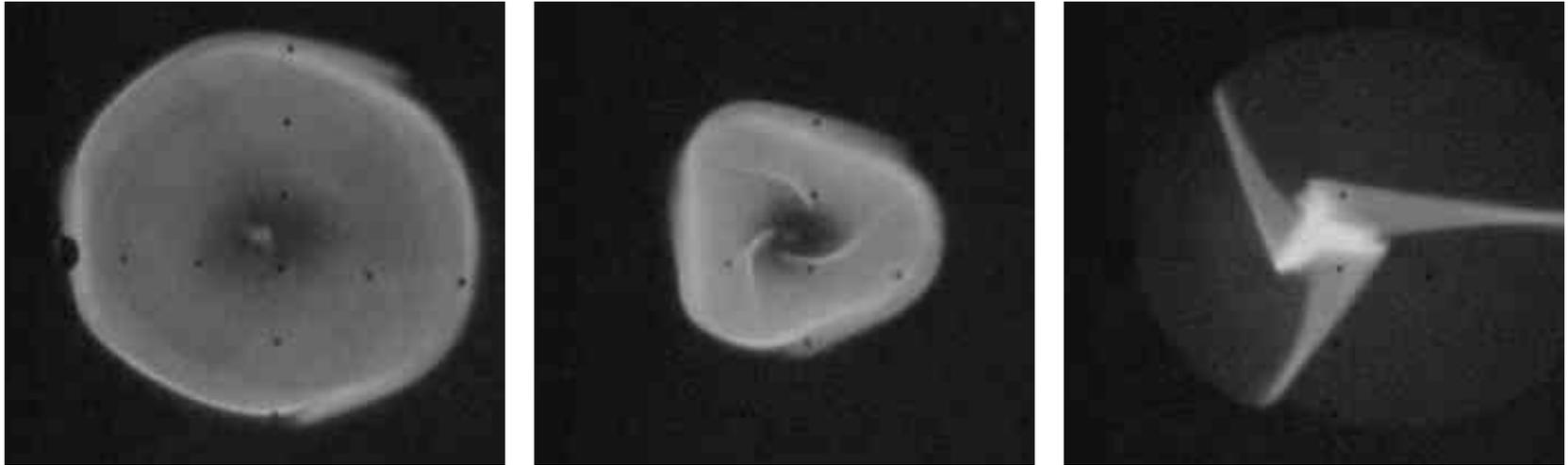
Measured beam profiles from CAPRICE at location B with increasing focusing strength of the beam line solenoid. Only one  $m/q$  is visible, all other are de- or over focused.
