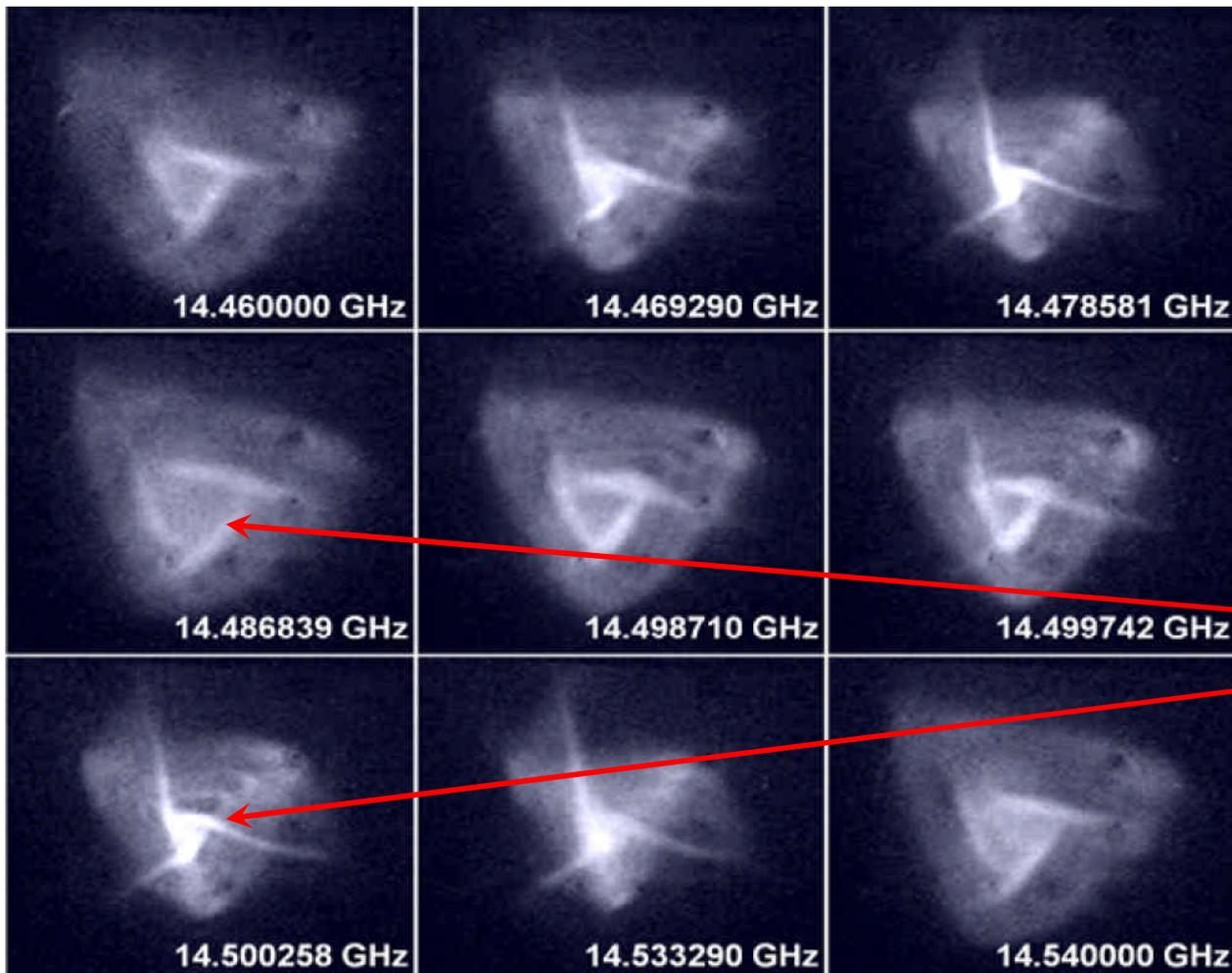
Viewing target directly behind extraction, before the beam line solenoid. Variation of frequency favors different modes. See the talk given by Luigi Celona (INFN Catania).
