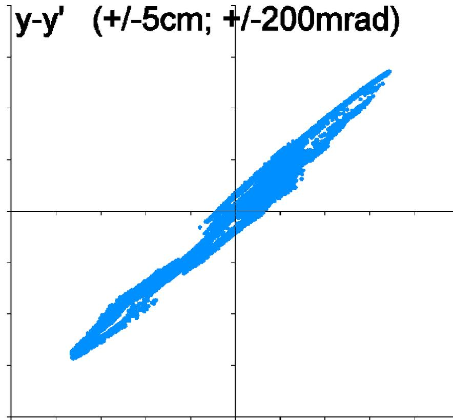
beam properties after extraction: vertical emittance.
