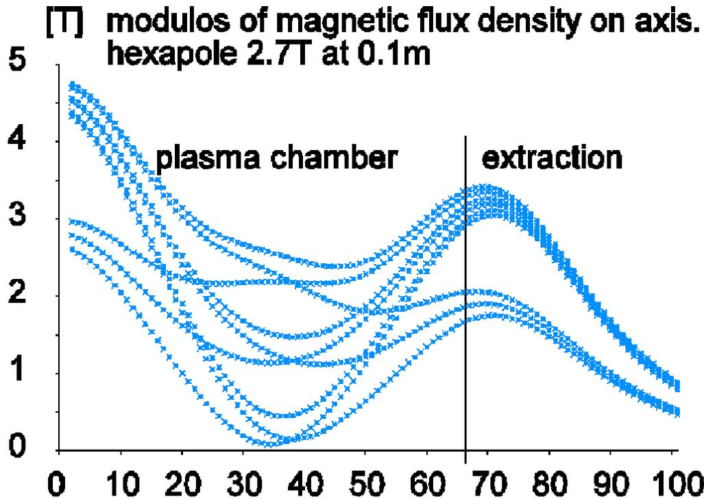
magnetic flux density on axis for different coil settings:
