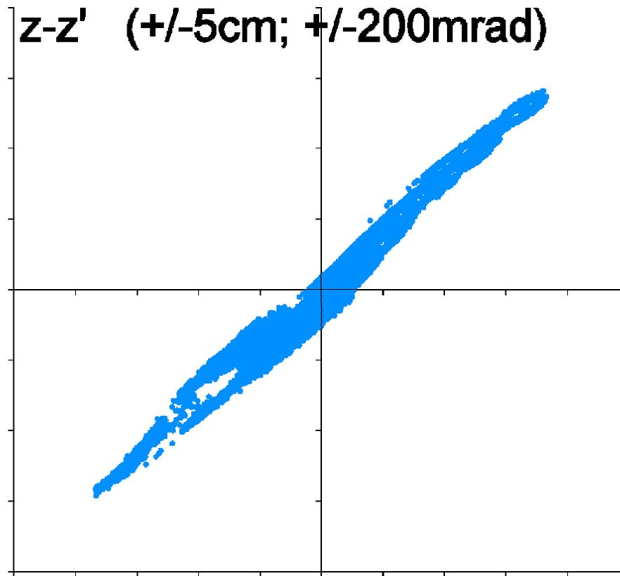
beam properties after extraction: horizontal emittance.
