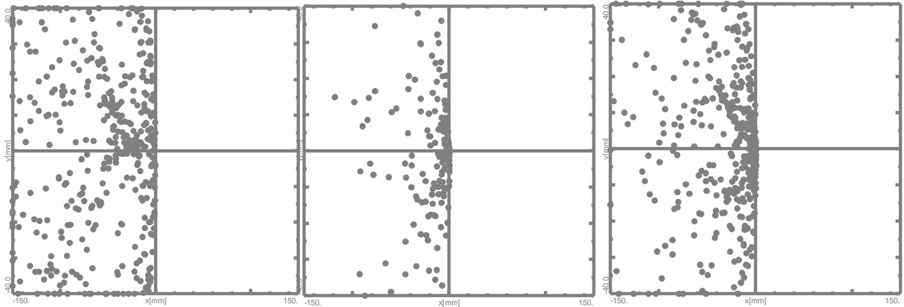
Real space distribution behind the dipole for different magnetic settings. vertical  $\pm 40\text{mm}$ , horizontal  $\pm 150\text{mm}$
