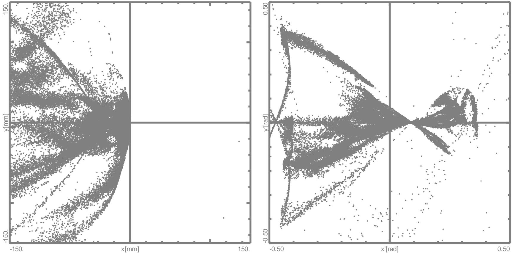
Real space distribution ( $\pm 150\text{mm}$ ) and momentum space ( $\pm 500\text{mrad}$ ) behind the dipole.
