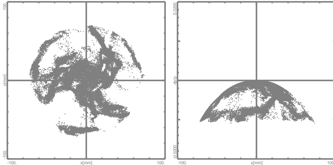
Real space distribution ( $\pm 100\text{mm}$ ) and horizontal momentum distribution ( $\pm 100\text{mm}$ ,  $\pm 20\text{mrad}$ ) behind the beam line solenoid.
