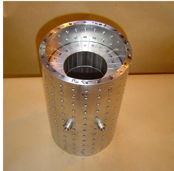
**Figure 4.** View of partially assembled Halbach sextupole magnet showing the individual magnet blocks.
