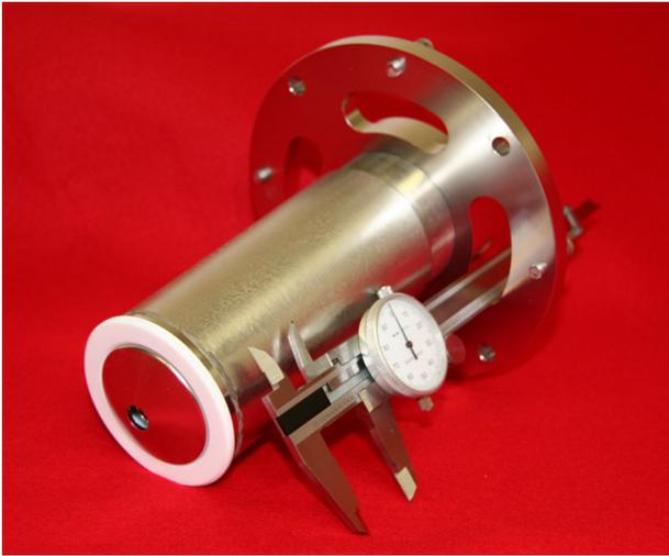
**Figure 12.** Extractor assembly of the charge-breeder source. The puller electrode is isolated from ground by the white Macor insulator and can be biased up to  $-2$  kV with respect to ground.
