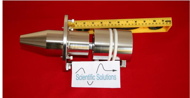
**Figure 20.** Ground shield (left) and first Einzel lens (right) in the injection line.
