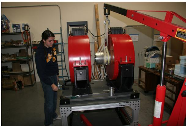
**Figure 9.** Installation of the high voltage assembly in the charge-breeder solenoids.
