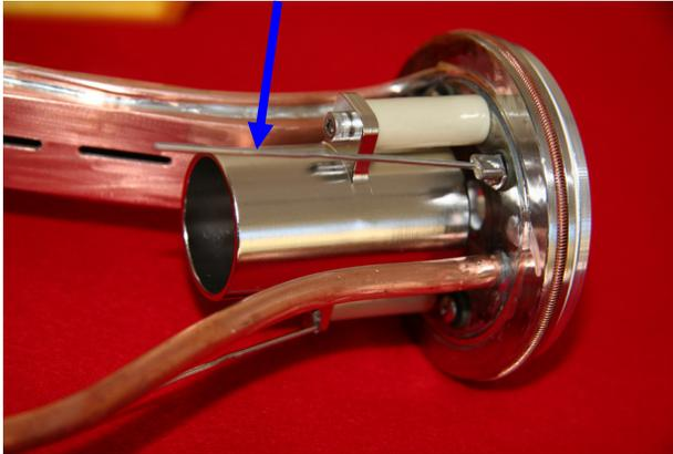
**Figure 18.** Detail of the plasma endwall assembly. The blue arrow denotes the voltage connection to the bias disk on the inside of the endwall.
