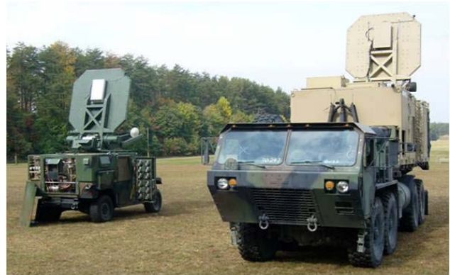
Figure 7: ADS system using a 100 kW, 95 GHz gyrotron
