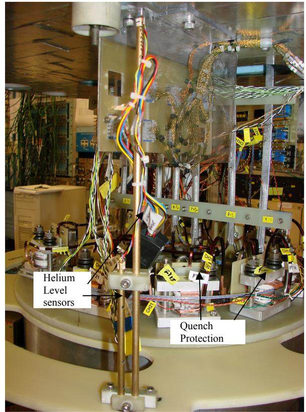
Figure 7: A detail view of the quench protection system, the vapor cooled leads and the diagnostic wiring.
