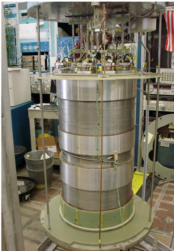
Figure 6 The VENUS magnet assembled for the cold test at the LBNL superconducting magnet test facility.
