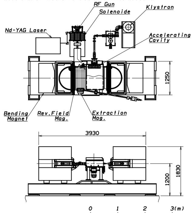
Figure 1: Top view of 150-MeV RTM with RF gun in injection system.
