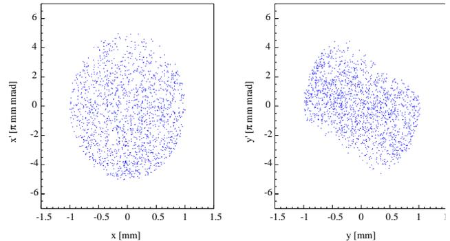
**Figure 2: Initial emittance of input beam from RF**
