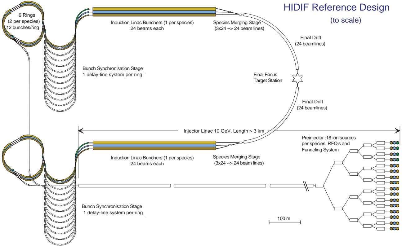
Figure 1: Layout of the HIDIF reference design
