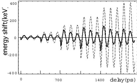
Figure 3: Calculated energy shift of a test bunch at  $n_p = 9.1 \times 10^{11} \text{cm}^{-3}$ . Dashed curve: in a homogeneous plasma. Solid curve: in the plasma density distribution shown by the dot-dash curve in Fig. 2.
