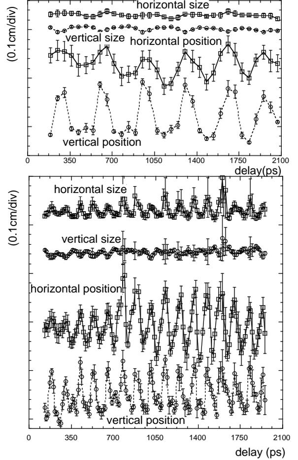
Figure 4: Delay dependence of horizontal and vertical shifts, and, horizontal and vertical sizes of test bunches at the energy analyzer. Plasma densities are  $1.0 \times 10^{11} \text{cm}^{-3}$  and  $9.1 \times 10^{11} \text{cm}^{-3}$  in the upper and lower figures, respectively. Injection timing of a drive bunch is every 350ps, with the first one at 0ps.
