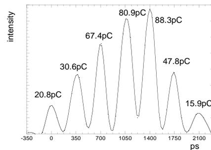
Figure 1: Bunch distribution in a drive beam. Total charge is 352pC. Bunch spacing is 350ps.
