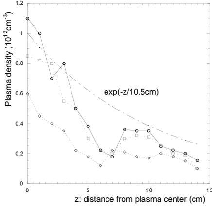
Figure 2: Plasma density distributions in a plasma chamber and their approximation used in the analyses.
