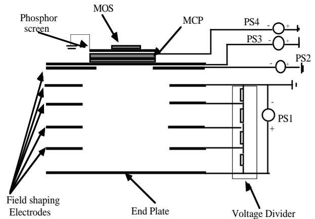
Fig.3 Electric scheme. PS1, PS2, PS3, PS4 are the Power supplies.
