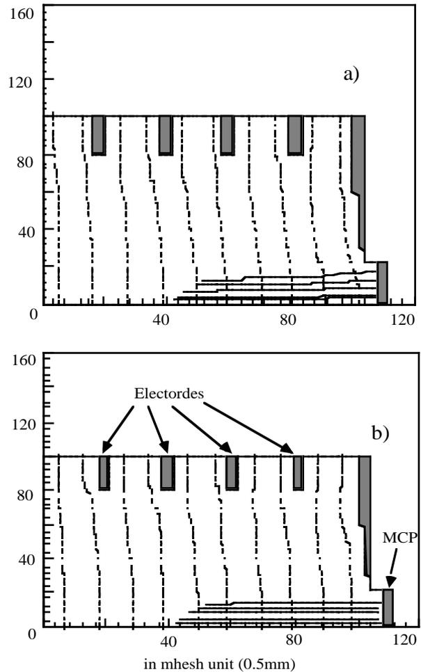
Fig.3 Trajectory simulation of residual gas ions with slightly different typical initial conditions.
