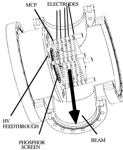
Fig.2 Mechanical design of the RG-BPM.
