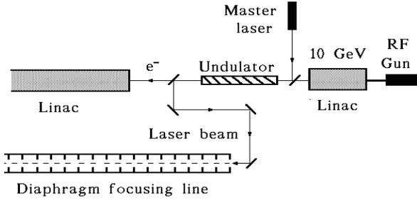
Figure 2: Conceptual scheme of an FEL amplifier for the photon linear collider at TESLA-500.
