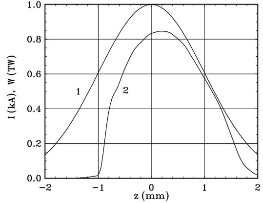
Figure 3: Axial distribution of the beam current in the electron beam (curve 1) and axial distribution of the output power in the optical beam (curve 2).
