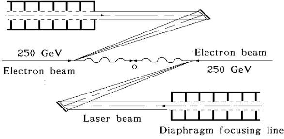
Figure 1: Conceptual scheme of the photon linear collider at TESLA-500.
