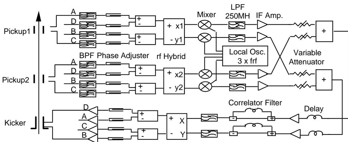
Figure 2. A block diagram of the transverse beam damping system
