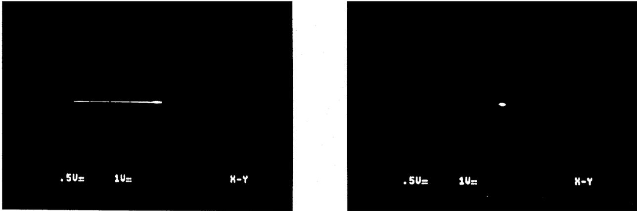
Figure 3. Photo of the oscilloscope showing damping of the horizontal oscillation before and after turn-on of the transverse damping system.
