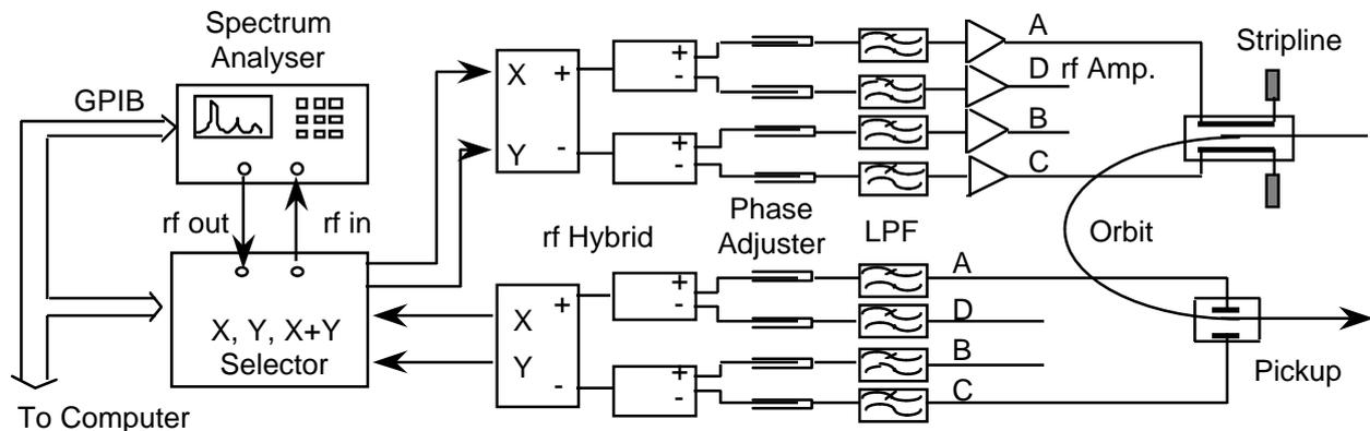
Figure 1. Schematic diagram of the tune measurement system
