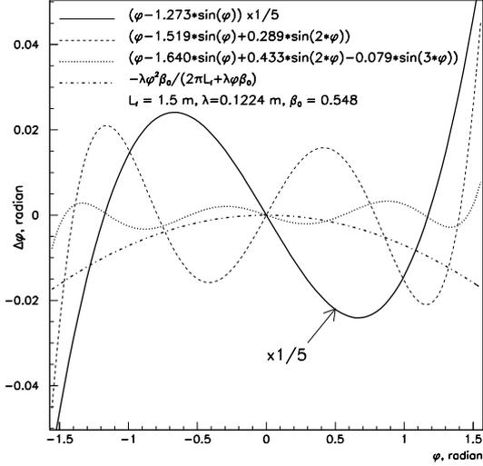
Figure 1: Deviation of particle phases from reference at longitudinal focus for  $N = 1, 2, 3$  harmonics. Parabola: error of linear approximation.
