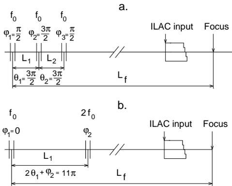
Figure 2: Schematic view of two prebuncher variants ( $f$ -frequency,  $\varphi$ -rf phase,  $\theta$ -transit angle).
