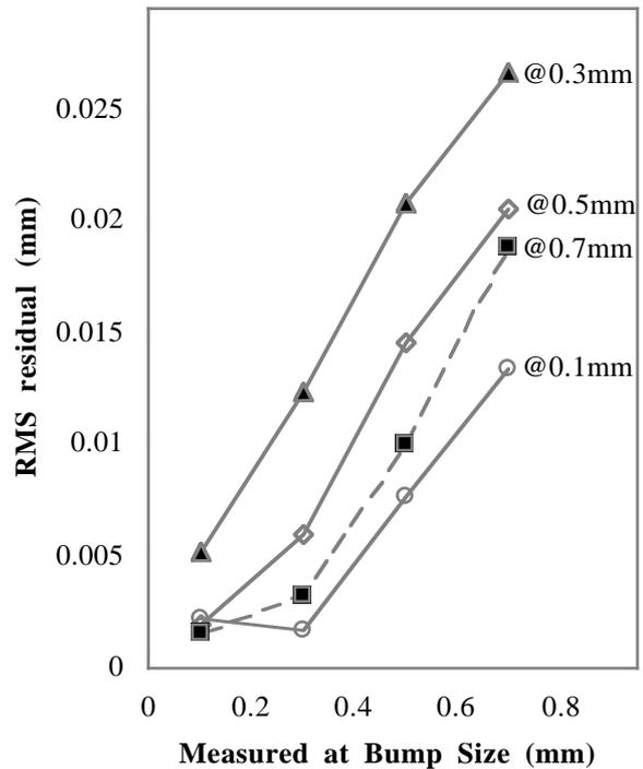
Figure 3: RMS residual at the TVMs (excluding TVM in bump) measured at different applied bump sizes for bump ratios optimised at 0.1mm, 0.3mm, 0.5mm and 0.7mm
