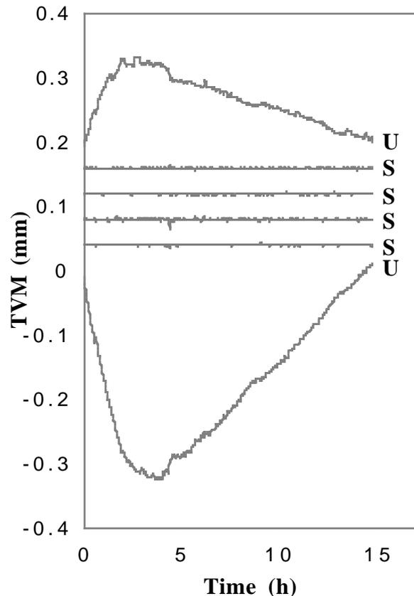
Figure 1: Comparison of servoed (S) and unservoed (U) beamlines over 15 hours of user beam. Note that an arbitrary constant has been added to each curve for display purposes: servoed TVMs remain close to  $0\mu\text{m}$  or, if stipulated, some other constant position.
