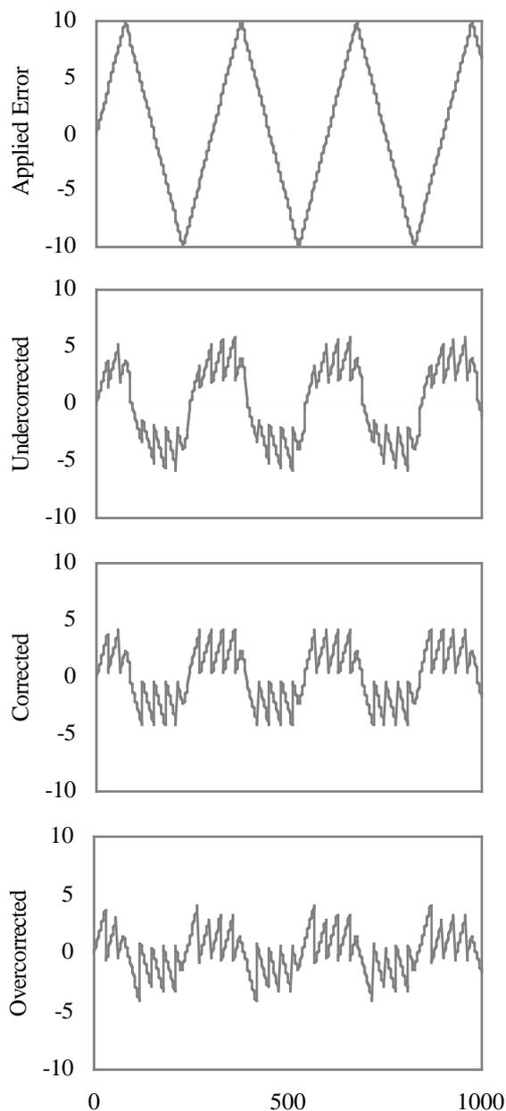
Figure 4: Induced oscillation and simulated servo performance for under-correction, exact (100%) correction and over-correction; horizontal axis shows time (s)
