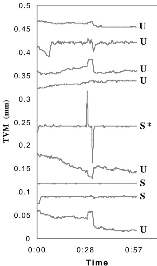
Figure 2: Comparison of servoed (S) and unservoed (U) beamlines showing correction of deliberately induced disturbance on a single servoed line (S\*)
