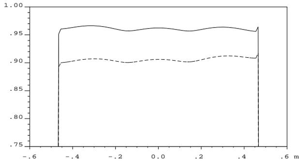
Fig. 3: MAFIA plot of normalized  $V_e(z)$
