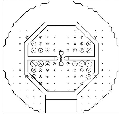
Fig. 5: MAFIA plot of the magnetic field in a transverse section in the middle of a ring
