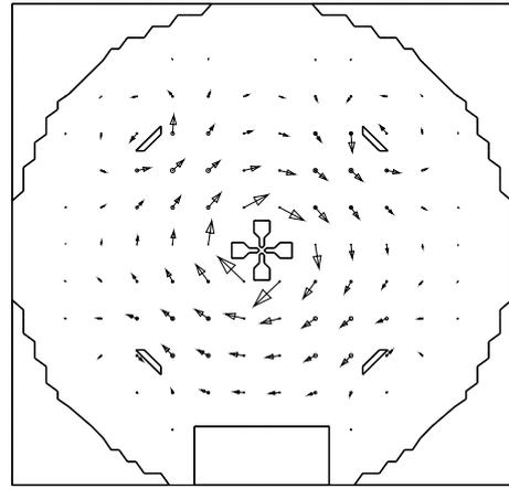
Fig. 4: MAFIA plot of the magnetic field in a transverse section in the middle of a cell
