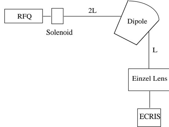
Fig. 1. Layout of extraction beamline of 18 GHz ECR ion source.
