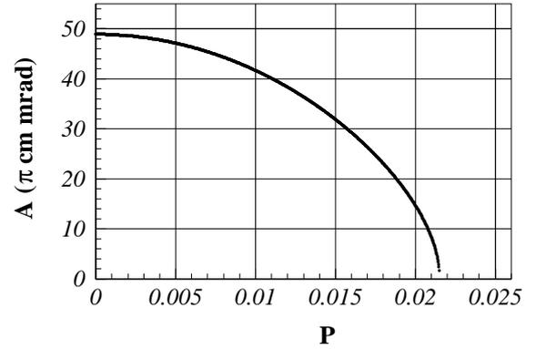
Fig. 2. Acceptance of the channel  $A$  as a function of space charge parameter of the beam  $P = \sqrt{2I/(I_0 \beta^3 \gamma^3)}$ .
