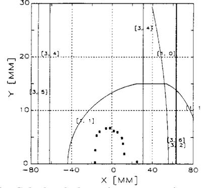
Fig. 3. Calculated dynamic aperture in comparison with limitations estimated in the single resonance approximation.
