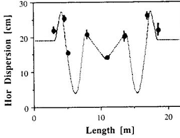
Fig. 4. Measured horizontal dispersion for the DDoptics. Circles: average over the same BPM family. Bars: one standard deviation.
