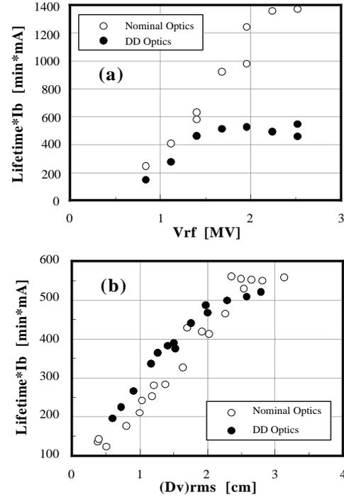
Fig. 6. Product of measured lifetime and average beam current versus (a) the RF voltage and (b) rms vertical dispersion  $(D_v)_{rms}$  at  $V_{rf} = 1$  MV, for the two optics, respectively.
