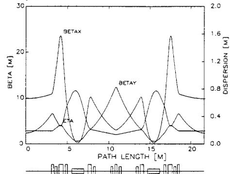
Fig. 1. Betatron and dispersion functions over a single cell of the DD optics considered in this work.
