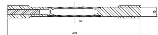
Fig. 2 Insertion device vessel - height of 15mm
