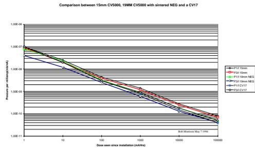
Fig. 6 Pressures on 15mm and 19mm ID vessels
