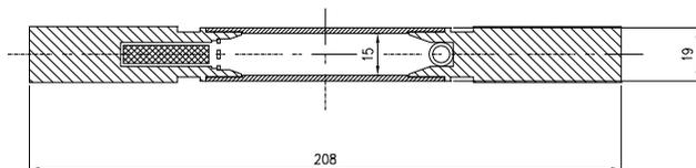
Fig. 1 Five meter long vacuum vessel - height of 19mm
