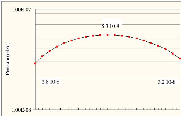
Measurements of pressure distributions are given without beam conditioning. **Figure 5** shows consequences of this conditioning. Results obtained with the above mentioned processes can certainly be improved, in this case, the oxygen and hydrogen levels in the metal have to be reduced.
