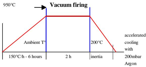
Fig. 3 Vacuum firing cycle
