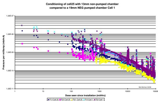
Fig. 5 Conditioning on the ID vessels
