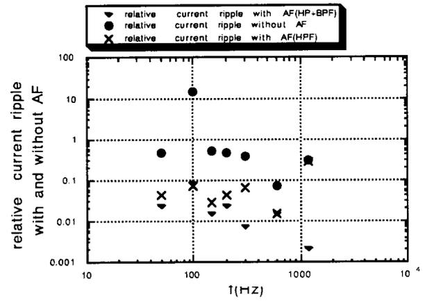
Figure 9: Relative current ripple with and without Active filter (normalized by the maximum current, rms)
