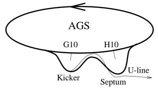
Figure 3: Schematic of the extraction orbit.
