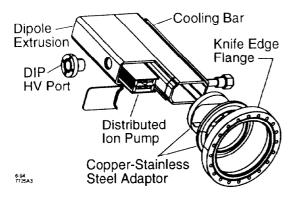
Figure 2 Isometric view of HER dipole vacuum chamber
