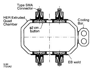
Figure 5 Cross section of quadrupole chamber showing BPM feedthroughs.
